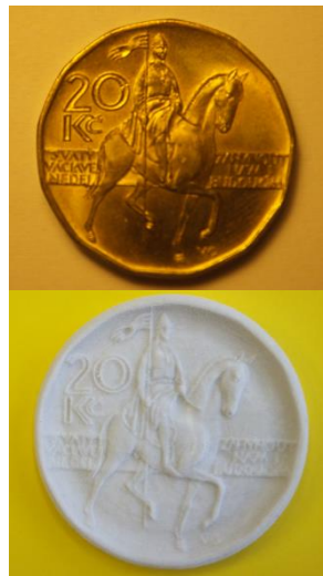
Figure 5. Coin scanned and 3D print of the reconstructed coin
