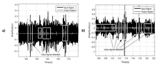
Figure 2 Voice detection areas in the "tabst\_B.wav", signal contaminated with pink noise. Input SNR - 5dB.
